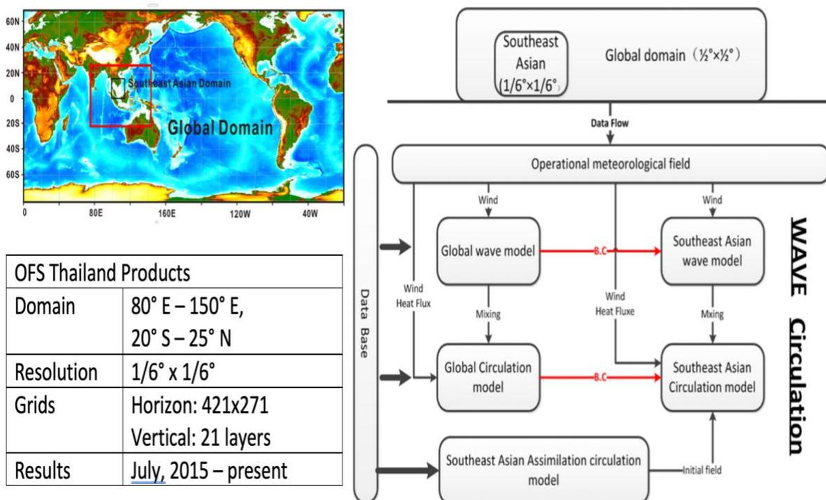
Figure 2: OFS simulation domain (Left) and framework (right)
