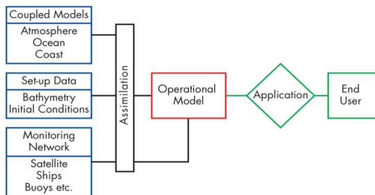
Figure 1: Components of a modelling simulation system
